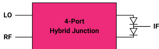
Fig. 5: Single balanced mixer with 4-port hybrid junction.
