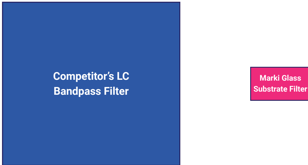
Fig. 1: To-scale footprints of competing low frequency filters.
